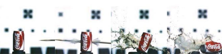
Selection of images taken from a 4,000 frames per second recording, with a 25 microsecond shutter (two microsecond shuttering is possible), of an arrow piercing a soda can. These images clearly show the arrows 'wobble' as it deflects inside the can.
