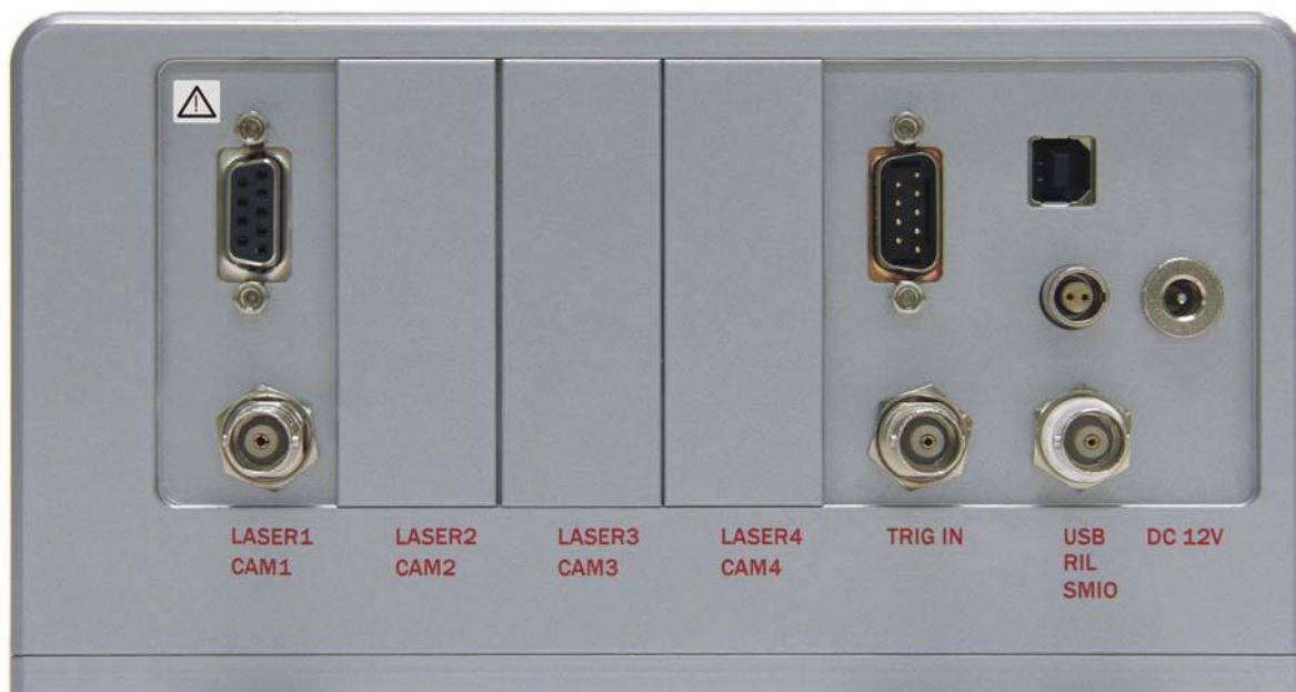
Fig. 3.3. Rear panel of CAVILUX Control unit.
