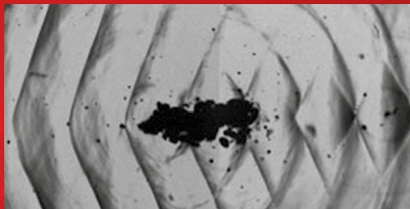
Shockwave formation in gel
