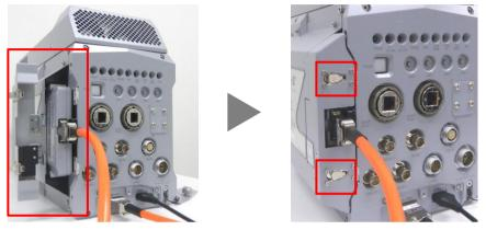
6. Connect the USB cable (type A) to the PC's USB 3.0 connector.
