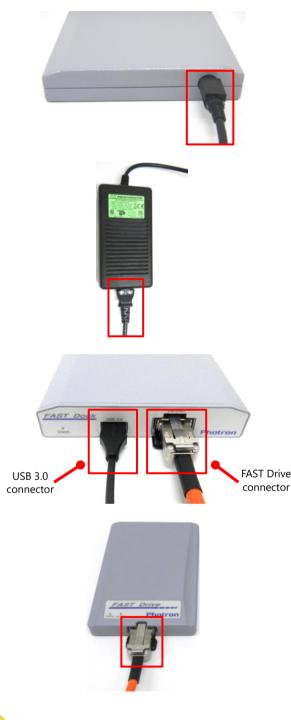
1. Connect the AC power supply adapter to the rear of the FAST Dock.
