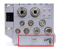
1. Remove the FAST Drive slot cover on the rear of the camera.
