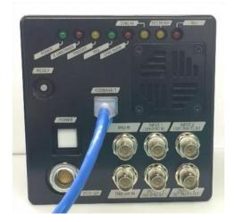
Insert a LAN cable to "1000BASE-T" connector.
